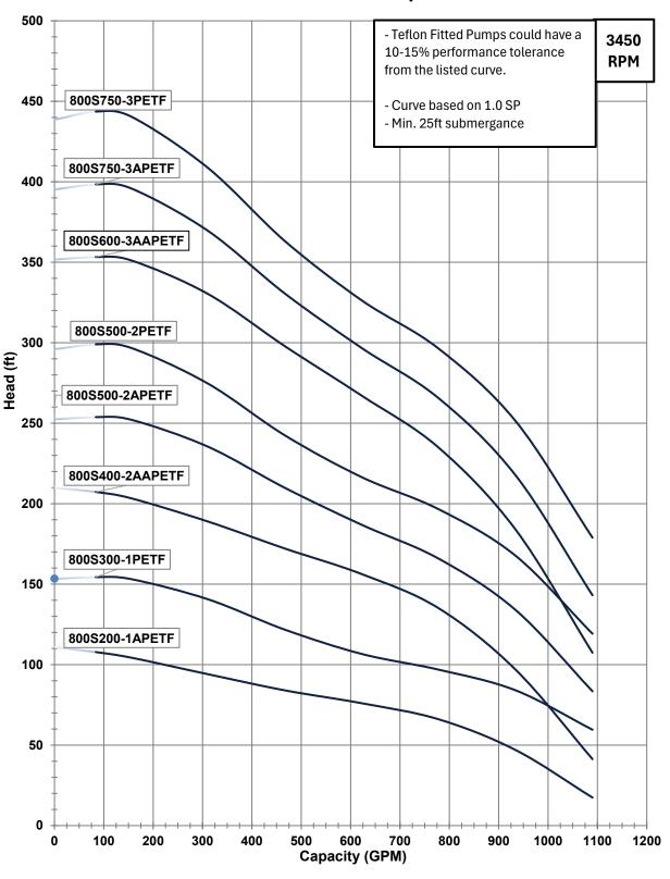
800S Teflon Fitted Pump Ends
