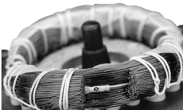
PTC sensor incorporated in winding
