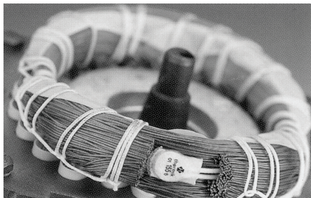
Thermal switch incorporated in winding
